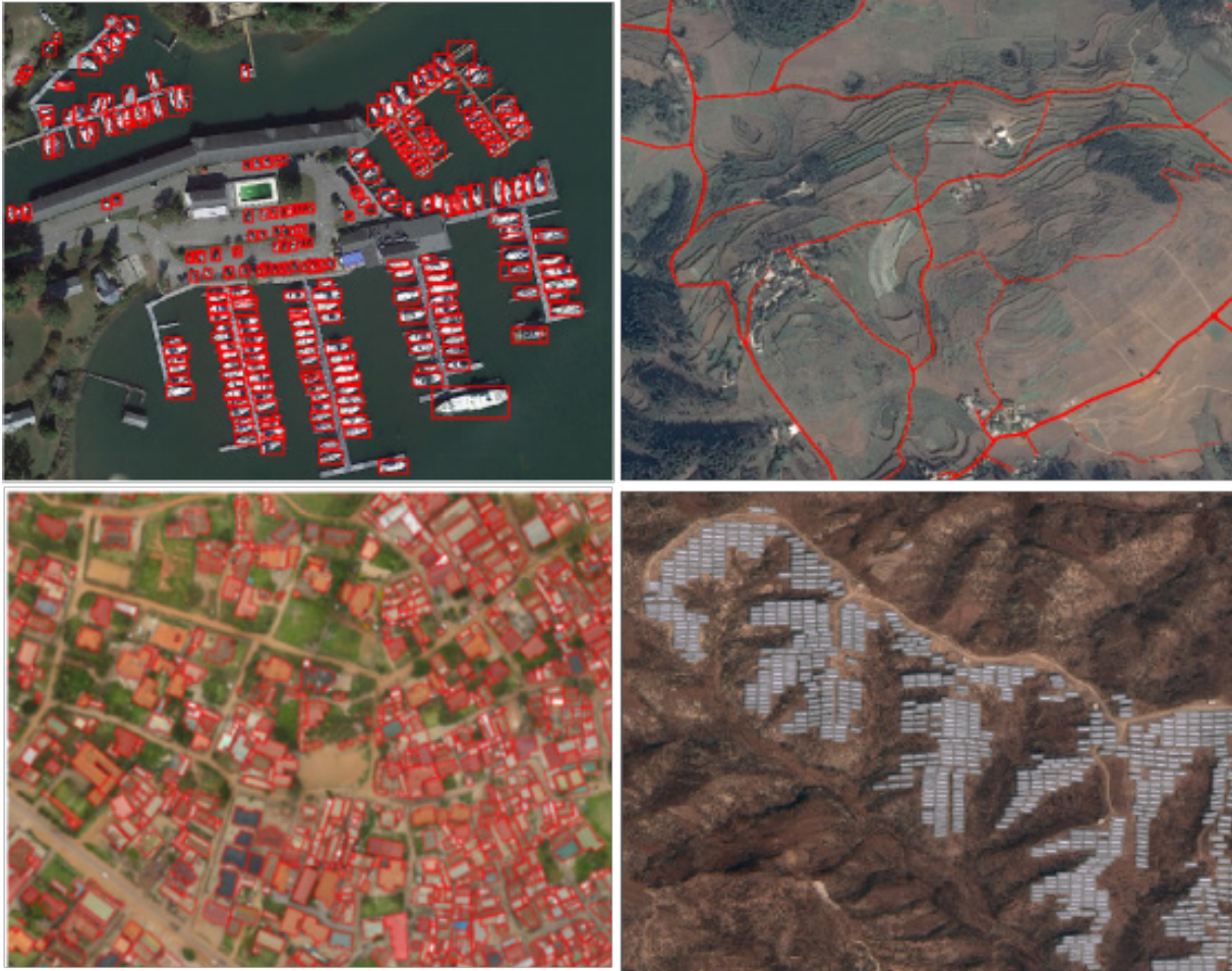
Extraction of basic geographic entities: ship and vehicle extraction (upper left); road extraction (upper right); building extraction (lower left); photovoltaic panel extraction (lower right)
